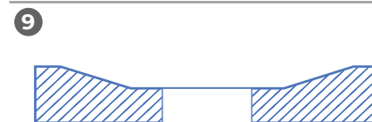
Grinding Wheels Recessed on One Side
